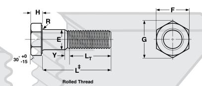
‡Length of a structural bolt is measured from the underhead bearing surface to the extreme end of the bolt.
